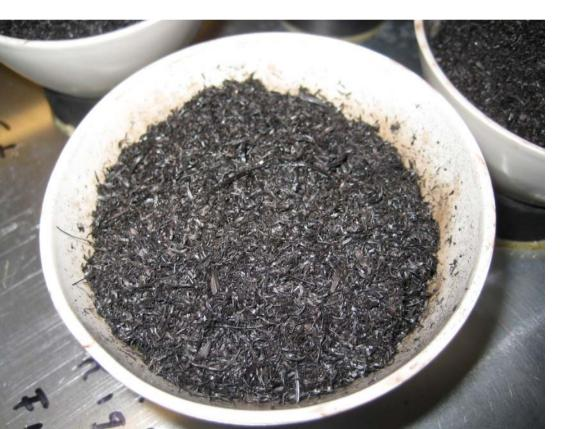
We are investigating the effect of formation conditions on the properties of biochar (from cellulose, lignin, pine, poplar, and switchgrass) and their implications for use of biochar as a soil amendment and for longterm carbon sequestration. **Properties related to** charring temperature and duration include changes in biochar yield, elemental composition, functional groups by NMR spectroscopy, surface area, and acid functional groups.
